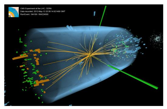
**Figure 1.** Event recorded with the CMS detector in 2012 at a proton-proton centre of mass energy of 8 TeV. The event shows characteristics expected from the decay of the SM Higgs boson to a pair of photons (dashed yellow lines and green towers). The event could also be due to known standard model background processes.
