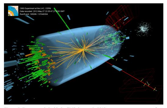
**Figure 2.** Event recorded with the CMS detector in 2012 at a proton-proton centre of mass energy of 8 TeV. The event shows characteristics expected from the decay of the SM Higgs boson to a pair of Z bosons, one of which subsequently decays to a pair of electrons (green lines and green towers) and the other Z decays to a pair of muons (red lines). The event could also be due to known standard model background processes.
