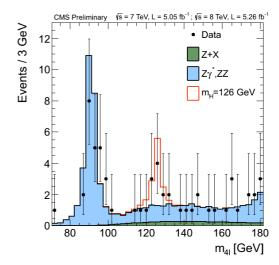
**Figure 4.** Distribution of the four-lepton reconstructed mass for the sum of the 4e,  $4\mu$ , and  $2e2\mu$  channels. Points represent the data, shaded histograms represent the background and un-shaded histogram the signal expectations. The distributions are presented as stacked histograms. The measurements are presented for the sum of the data collected at centre of mass energies of 7 TeV and 8 TeV.
