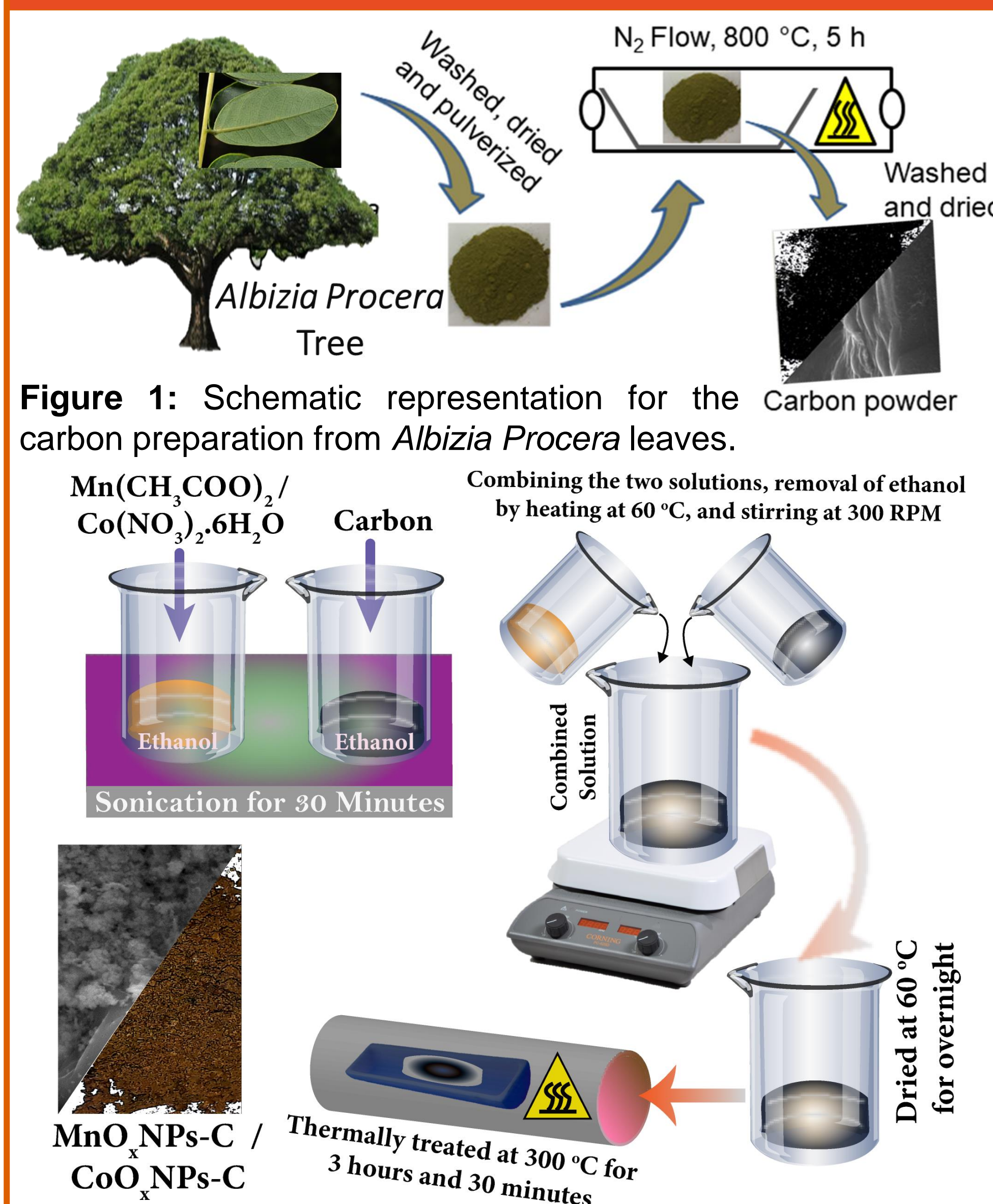
Figure 2: Schematic showing the sample preparation of manganese oxide / cobalt oxide and carbon nanocomposite.
