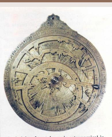
The height of pretelescopic astronomical instrument development was the refinement of astrolabes, used to show the positions of the Sun and stars for any time and date. This example dates from 1628 and was made by a family of astrolabe makers in Lahore (now in Pakistan). Courtesy Owen Gingerich.
