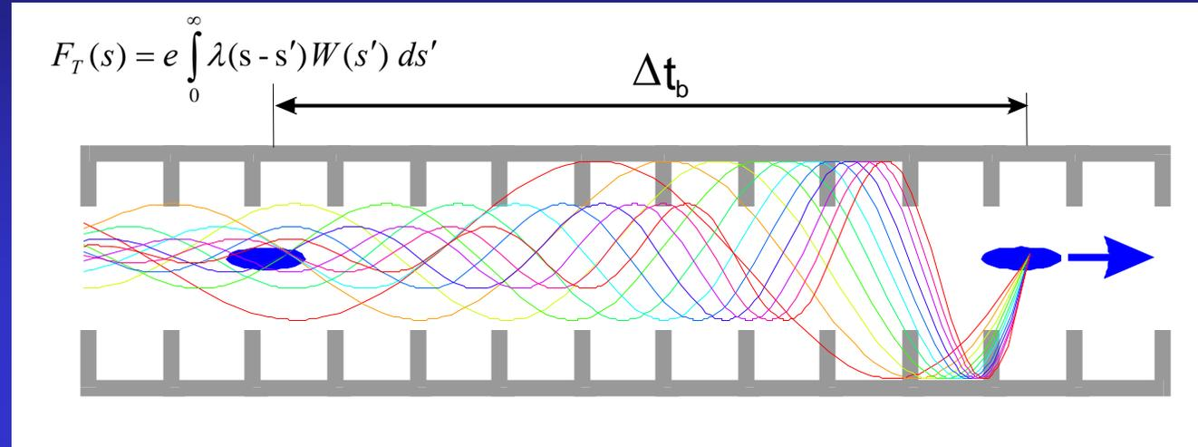
Bunch current generates transverse deflecting modes when bunches are not on cavity axis.
