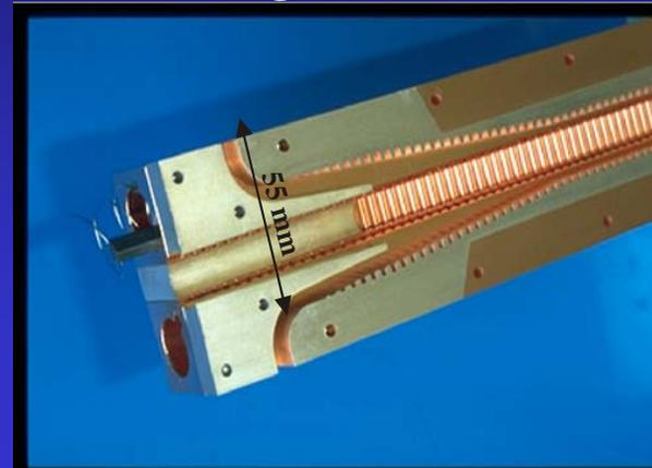
30 GHz accelerating structure of CTF II main beam
