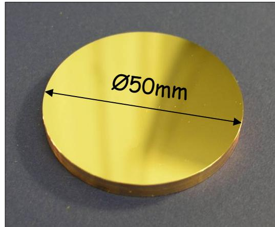
Diamond turned test sample, Ra 0.025 $\mu$ m
