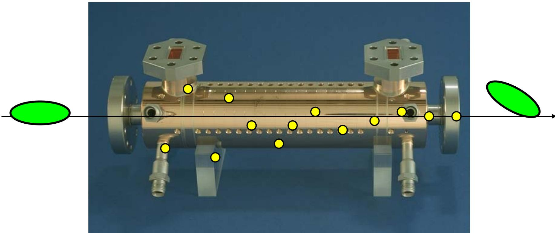
**Short-range transverse wakefields:** Misalignments, beam and structures, induce diffraction of field following relativistic bunch which acts back on itself causing it to grow in phase space (very, very higher-order modes) Effect shown in green.
