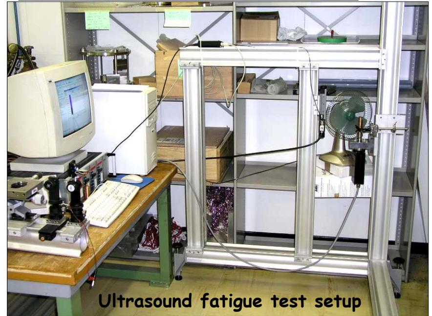
Ultrasound fatigue test setup
