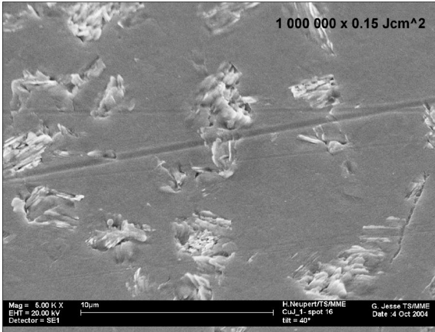
**Cu-OFE at  $10^6$  cycles,  $\Delta T=90^\circ\text{C}$
