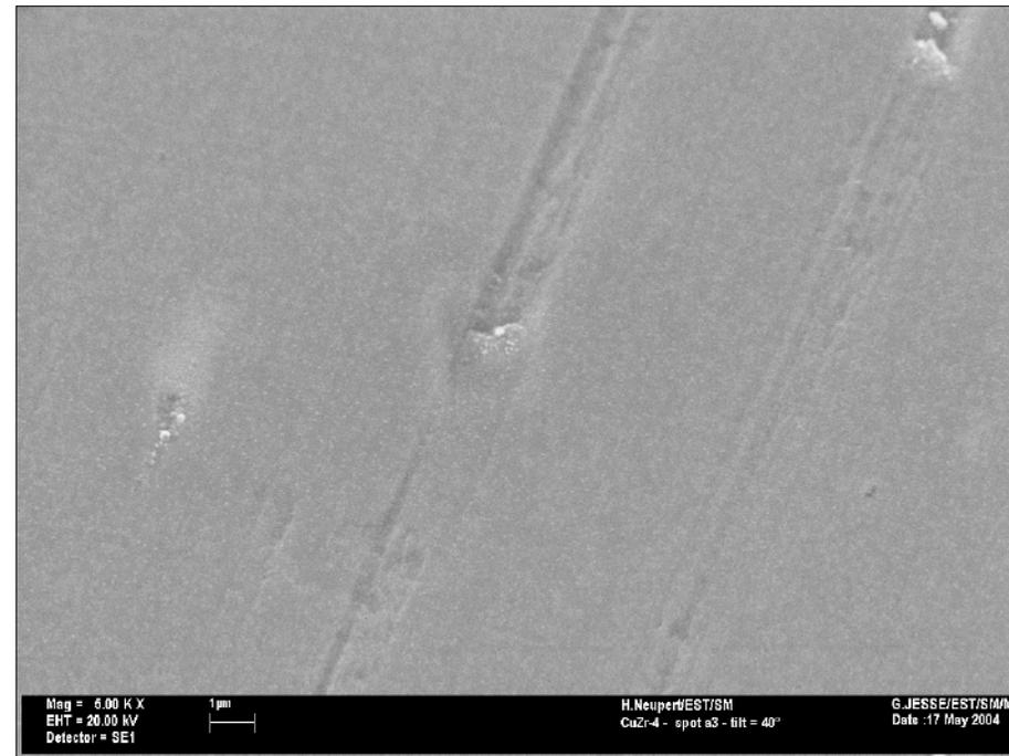
**CuZr at  $10^6$  cycles,  $\Delta T=90^\circ\text{C}$
